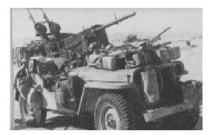
Desert Jeep modified by the SAS. Twin Vickers machine guns at the rear and a single Vickers and 0.5 Browning at the front. Note the water condenser on the front bumper. 3.
