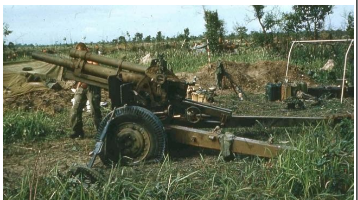
Bravo gun .. at Coral on the morning of May 13, 1968, with two blown tyres and damage to the gun trail
