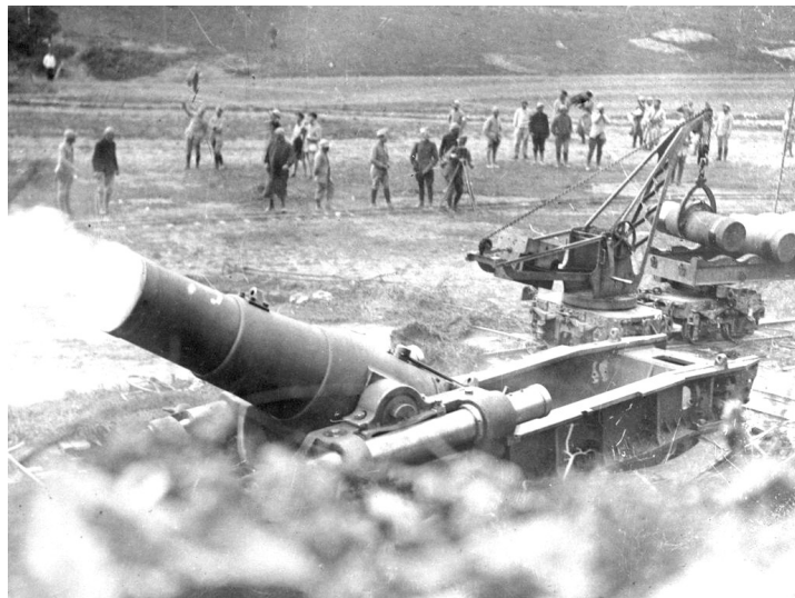
In the infamous Somme region of France, a French 270 millimetre mortar cannon bombards the German trenches, inspiring terror, destruction and lowering enemy morale. A crane needs to be used to transport the large ammunition rounds to feed this beast.
