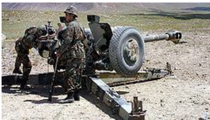
The D-30, or 122-mm howitzer D-30 is a Soviet Howitzer that first entered service in the 1960s. It is a robust piece that focuses on the essential features of a towed field gun suitable for all conditions. The D-30 has a maximum range of 15.4 kilometers, or over 21 km using RAP ammunition.
